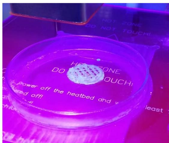
**Figure 8.** PLLA-based bioink produced.
