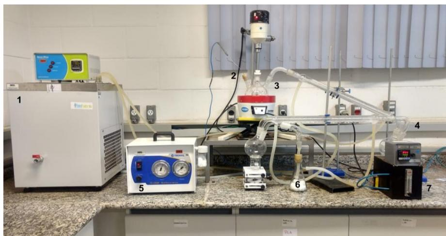
**Figure 3.** Experimental unit (1) water bath; (2) thermocouple; (3) main reactor with a heating mantle; (4) by-product reservoir; (5) vacuum-pressure pump; (6) trap; (7) thermal controller.
