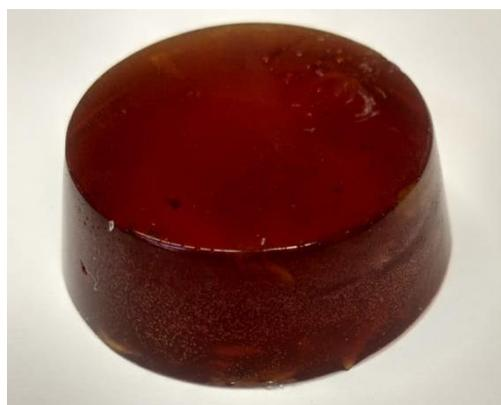
**Figure 4.** The raw PLLA produced.
