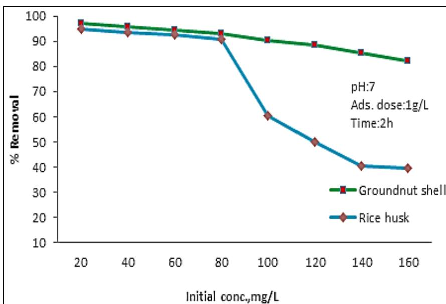
Fig. 3: Effect of Initial Concentrations on Lead Removal by Rice Husk and Groundnut Shell.
