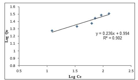
Fig. 15: Freundlich Isotherm for the Adsorption of Lead on to Combined Adsorbents.
