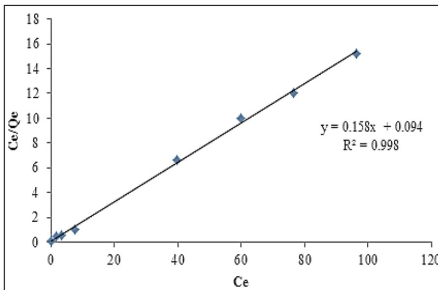
Fig. 7: Langmuir Isotherm for the Adsorption of Lead on to Rice Husk.
