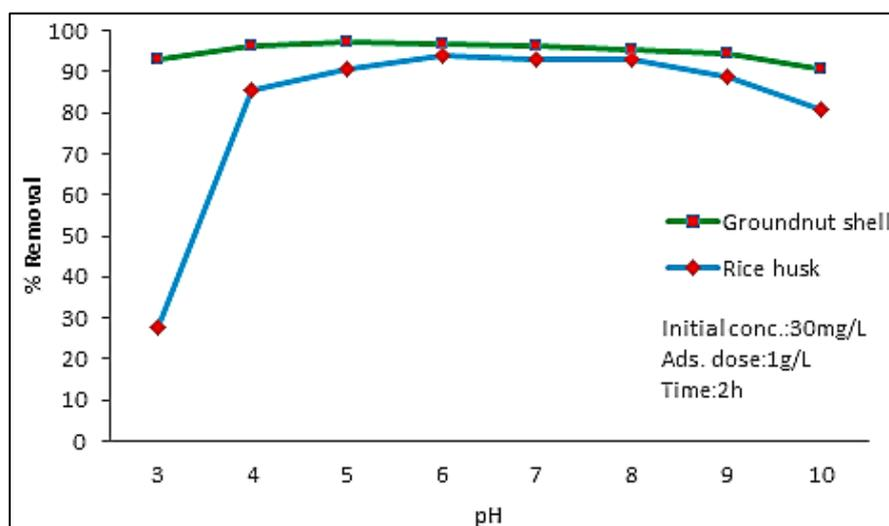
Fig. 1: Effect of pH on Lead Removal by Rice Husk and Groundnut Shell.
