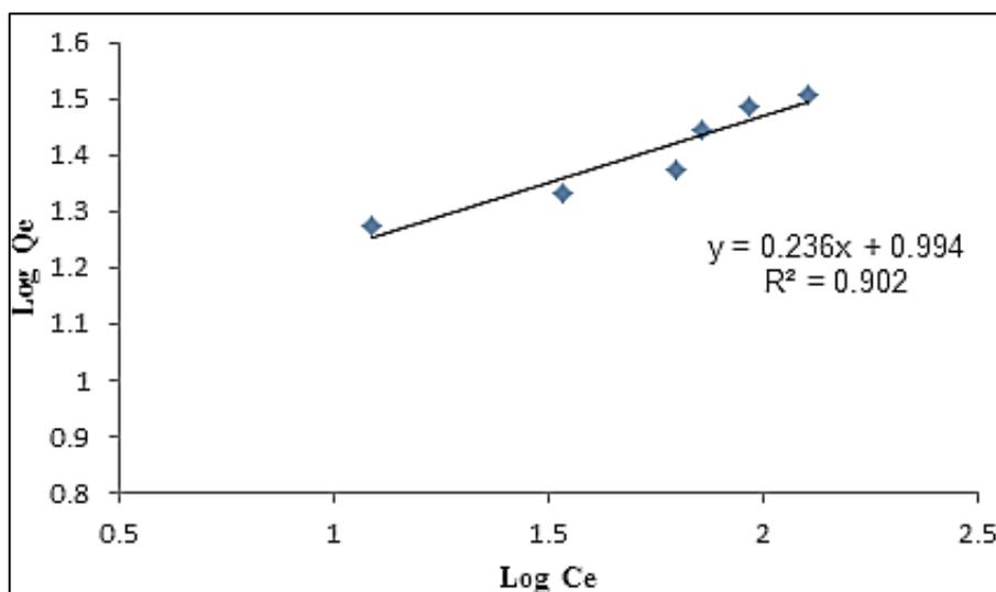
Fig. 15: Freundlich Isotherm for the Adsorption of Lead on to Combined Adsorbents.
