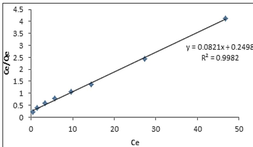
Fig. 9: Langmuir Isotherm for the Adsorption of Copper on to Rice Husk.
