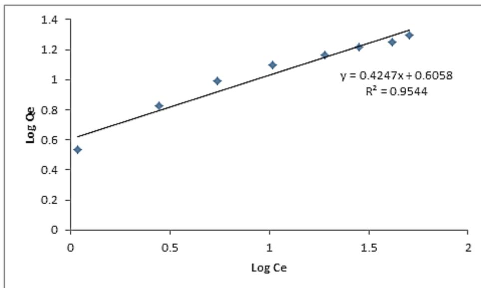
Fig. 17: Freundlich Isotherm for the Adsorption of Copper on to Groundnut Shell.
