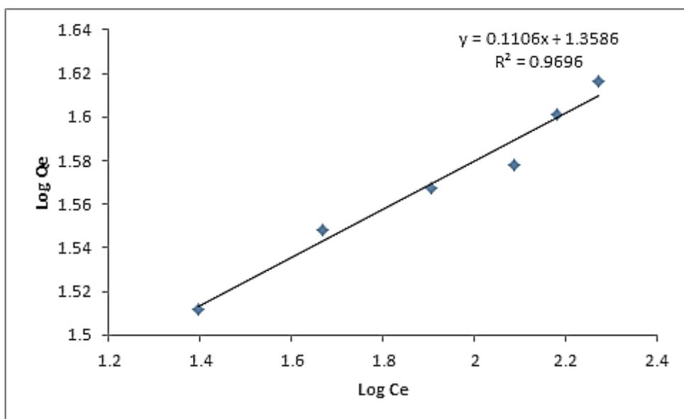
Fig. 18: Freundlich Isotherm for the Adsorption of Copper on to Combined Adsorbents.
