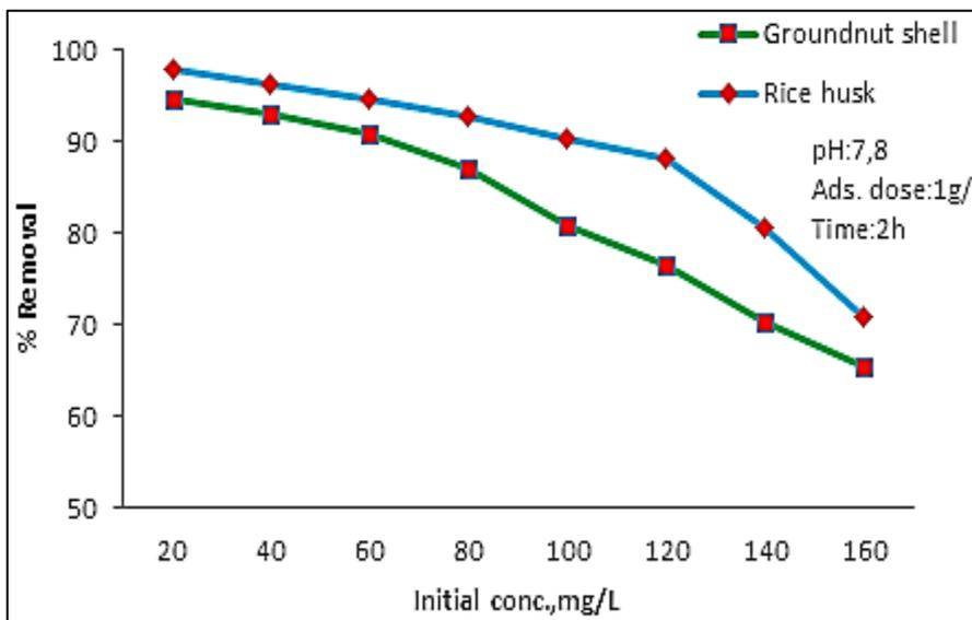
Fig. 4: Effect of Initial Concentrations on Copper Removal by Rice Husk and Groundnut Shell.
