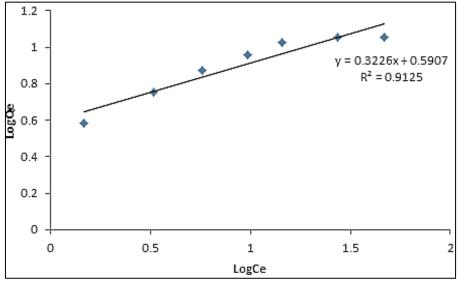
Fig. 16: Freundlich Isotherm for the Adsorption of Copper on to Rice Husk.
