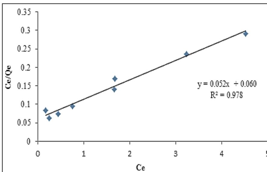
Fig. 8: Langmuir Isotherm for the Adsorption of Lead on to Groundnut Shell.
