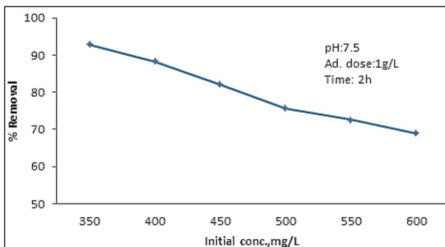
Fig. 6: Effect of Initial Concentration on Copper Removal by combined Adsorbents.
