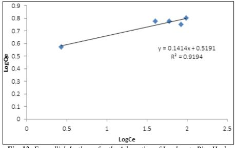
Fig. 13: Freundlich Isotherm for the Adsorption of Lead on to Rice Husk.
