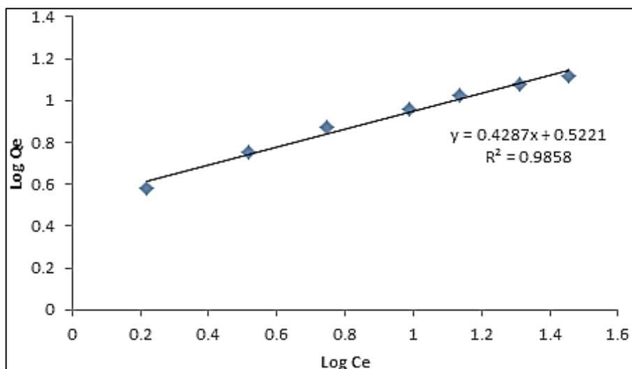
Fig. 14: Freundlich Isotherm for the Adsorption of Lead on to Groundnut Shell.
