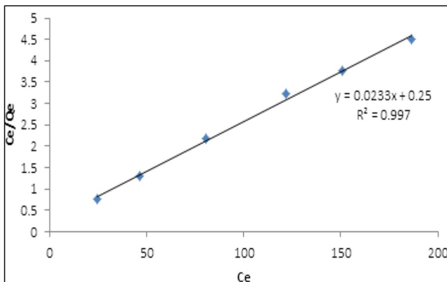
Fig. 12: Langmuir Isotherm for the Adsorption of Copper on to Combined Adsorbents.
