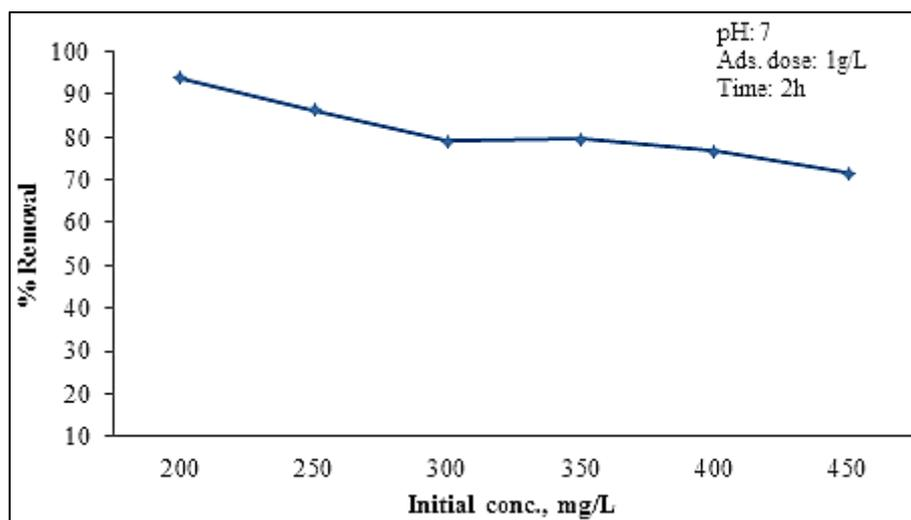
Fig. 5: Effect of Initial Concentration on Lead Removal by Combined Adsorbents.
