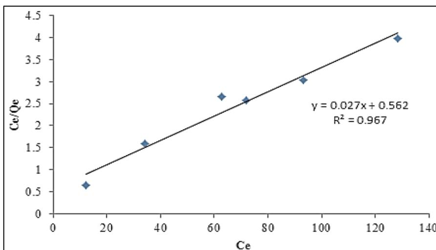
Fig. 11: Langmuir Isotherm for the Adsorption of Lead on to Combined Adsorbents.
