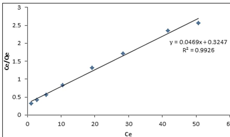
Fig. 10: Langmuir Isotherm for the Adsorption of Copper on to Groundnut Shell.
