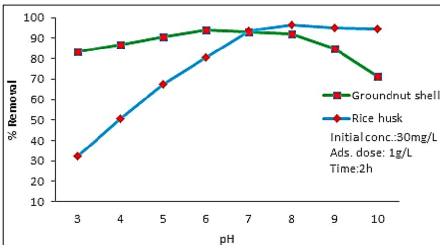
Fig. 2: Effect of pH on Copper Removal by Rice Husk and Groundnut Shell.
