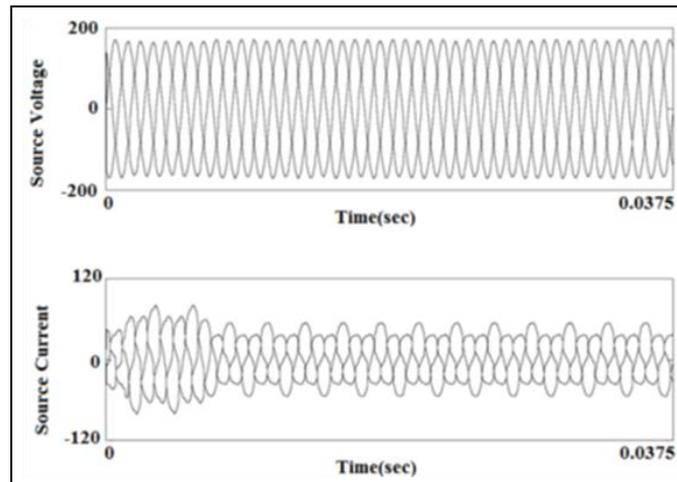
**Fig. 4:** Waveforms of an Uncompensated System (Source Voltage and Source Current).
