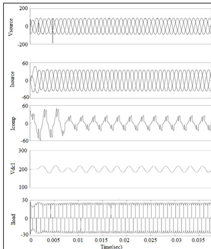
**Fig. 5:** Source Voltage, Source Current, Compensation Current (Phase B), DC Link Voltage and Load Current Waveforms of Active Power Filter Using Constant Instantaneous Power Control Strategy.
