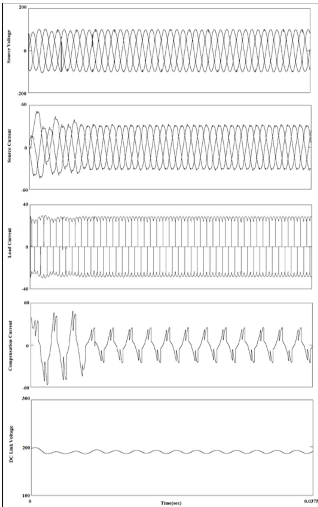
**Fig. 6:** Source Voltage, Source Current, Load Current and DC Link Voltage Waveforms of Active Power Filter using Constant Instantaneous Power Control Strategy using ANN and Genetic Algorithm with All Three Loads Connected to Aircraft System.
