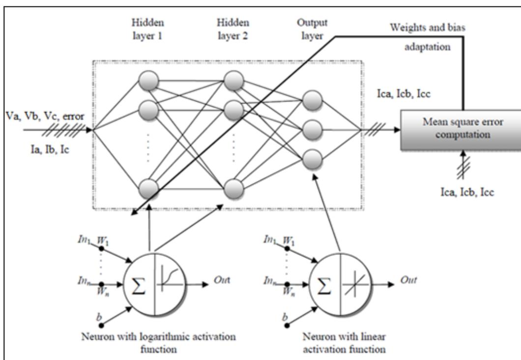
Fig. 3: Artificial Neural Network for Modeling.
