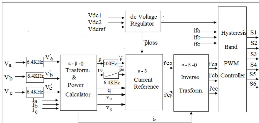
Fig. 2: Control Block Diagram of the Shunt Active Filter Using Constant Instantaneous Power Control Strategy.
