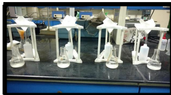
Fig. 5: Filtration of Samples with Whatman 42 Filter Paper.
