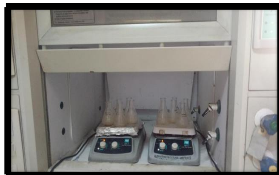
Fig. 4: Digestion of Soil Samples with Nitric Acid and Perchloric Acid.
